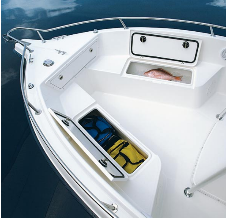
Forward area features twin fish/storage boxes with overboard drains.
